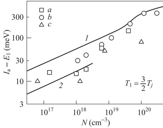
FIG. 4. Thermal ionization energy of boron atoms  $E_1 < I_a = 370$  meV at the temperature  $T_1 = 3T_j/2$  as a function of their concentration  $N$  in a  $p$ -type diamond. Calculations of  $E_1$  using Eq. (31) are shown by curves: 1 for  $K=0.15$  and 2 for  $K=0.5$ ; experimental data are shown by markers:  $a$ —Ref. 72,  $b$ —Ref. 73, and  $c$ —Ref. 80.
