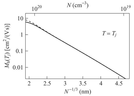
FIG. 6. Hopping drift mobility  $M_h(T_j)$  of holes via boron atoms in the charge states (0) and (–1) in a diamond crystal of  $p$ -type calculated using Eq. (34) as a function of boron concentration  $N$  at the temperature  $T = T_j$  for  $K = 0.15$ . Dashed line is the calculation of  $M_h(T_j)$  for  $N_h = (1 - K)KN$ .
