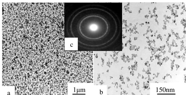
Figure 1. TEM images of the powder  $ZrO_2 + 3 \text{ mol.}\% Y_2O_3$ , (700°C, 2h) with magnification of 10 000 (a) 70 000 (b) and the characteristic pattern of the electron diffraction (c).
