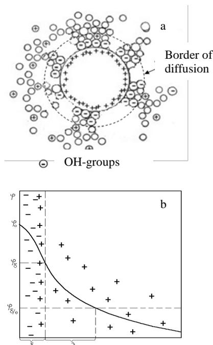
Figure 6. The electric double layer of  $ZrO_2$  particles (a) and change of its potential (b).
