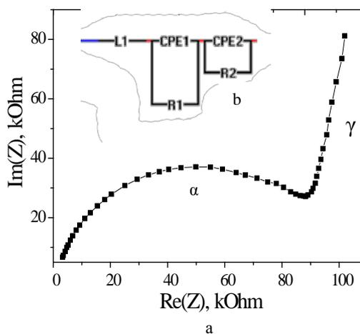
Figure 3. Hodograph of impedance of sample composition  $ZrO_2-3 \text{ \% } Y_2O_3$  (700 °C, 2h)
