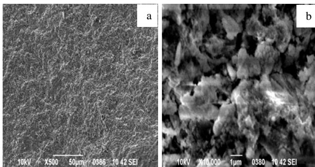
Figure 2. SEM images of fracture of compact sets (500 MPa) of the powder  $ZrO_2 + 3 \text{ mol.}\% Y_2O_3$  (700°C, 2h) with magnification of 500 (a) and 10 000 (b).
