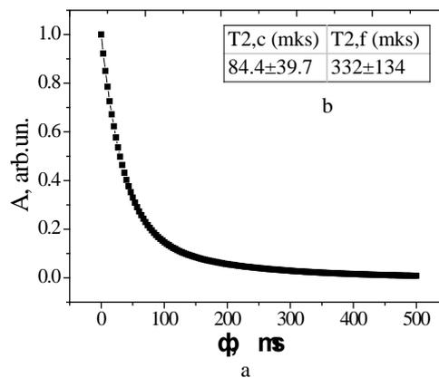
Figure 5. The experimental dependence of the damping of the spin-echo signal (a) and the values of the relaxation times of the magnetic moments of the hydrogen nuclei  $^1H$  (b)
