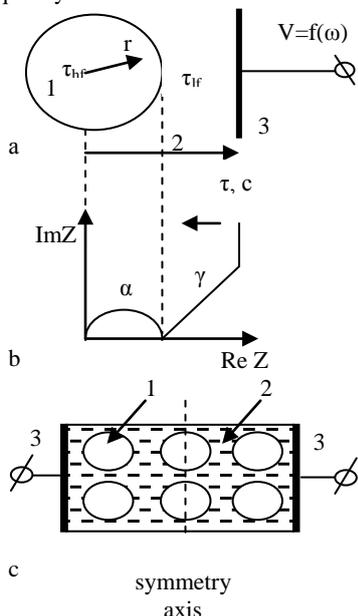
Figure 4. Geometric representation of nanopowder system with respect to the electrical properties (a); the spatial relationship (r) and time ( $\tau$ ) coordinate with the shape of the hodograph (b); model representation in accordance with the actual spatial distribution of the phase (c), where 1 - the volume of the dielectric nanoparticles; 2 - ion-conductive dispersion medium; 3 – electrode; r - radius vector;  $\tau$  - typical response time (time constant) of the structural elements).
